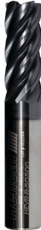
Helical Solutions' HEVR-SR five-flute, variable-pitch carbide end mill with AlTiN coating and a .030" corner radius.
