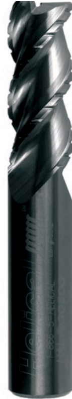
Helical Solutions’ HAL-C-SR three-flute carbide end mill. This tool has a serrated edge for breaking chips and is considered a roughing/semi-finishing tool.
