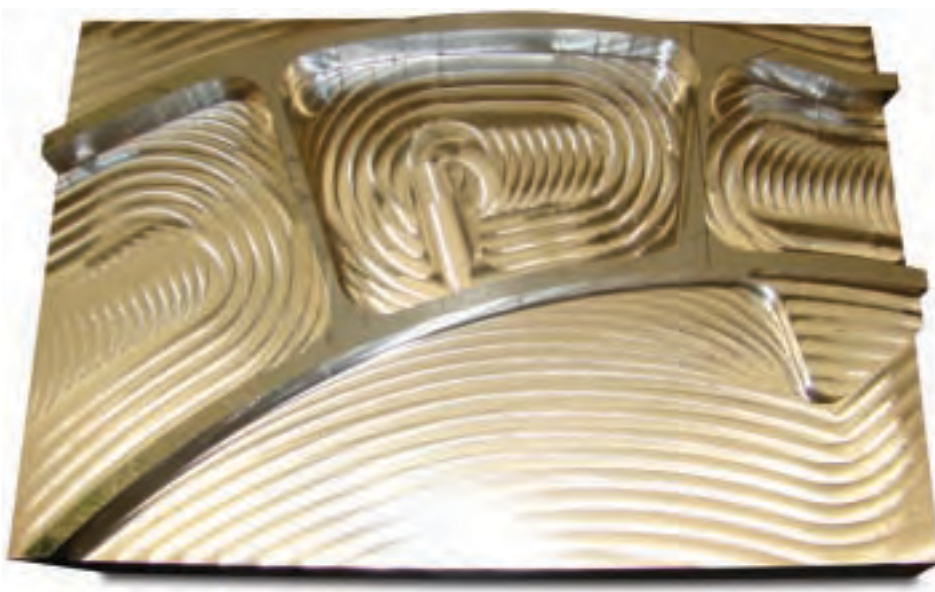
A completed 6061 aluminum part cut by a Helical Solutions’ HAL-C-SR three-flute carbide end mill with a Zirconium Nitride (ZrN) coating for improved lubricity and a VoluMill™ toolpath. This was achieved with an SFM of 1,560, RPM of 12,000, IPM of 1,000, and 100 CIM MRR.
