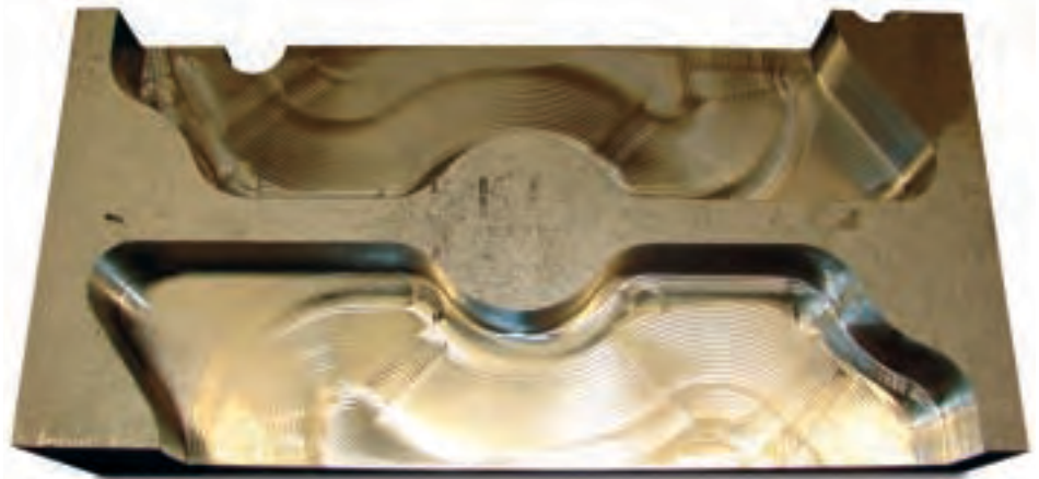
A completed 304 Stainless Steel part cut by a Helical Solutions HEVR-SR five-flute variable pitch carbide end mill with Aluminum Titanium Nitride (AlTiN) coating for heat resistance plus a .030" corner radius and a VoluMill™ toolpath. This was achieved with an SFM of 1,144, RPM of 8,800, IPM of 110, and 3.44 CIM MRR.
